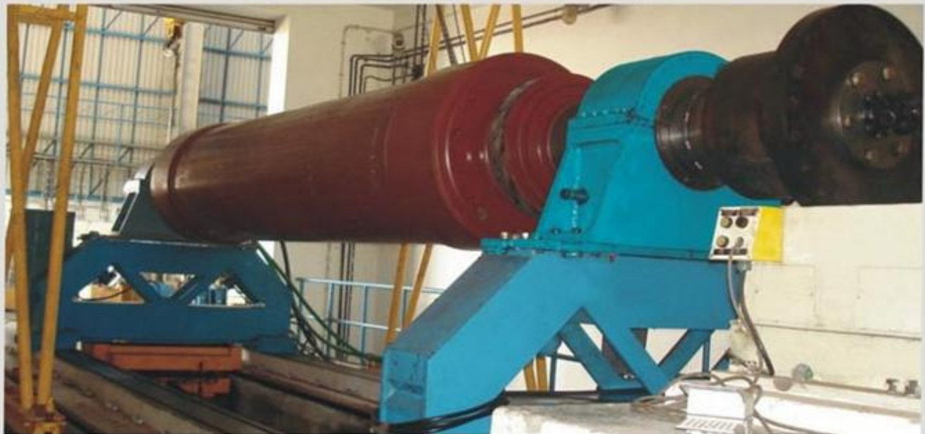
A 32 ton generator rotor being balanced at operating speed of 3000 rpm on ABRO HR25K machine
